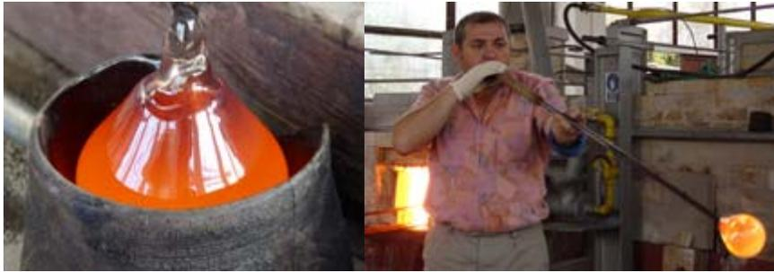
The glass ball at the end of pipe has to be formed using wooden tools, until is symmetrically shaped and this is the first time when air is blown into it.
