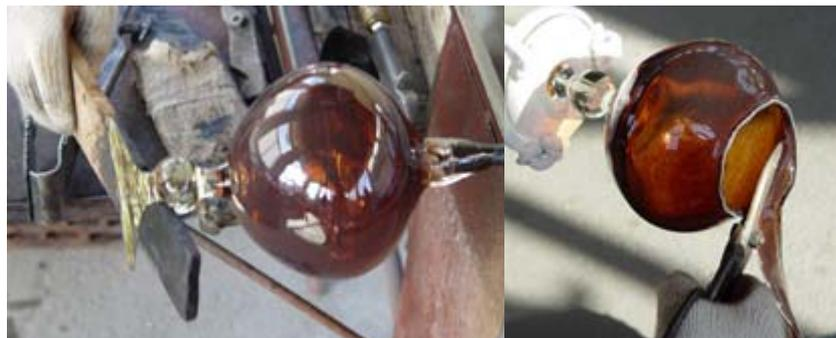
After the object is well shaped, the final adjustments has to be made (cutting, rewarming, opening, ...).
