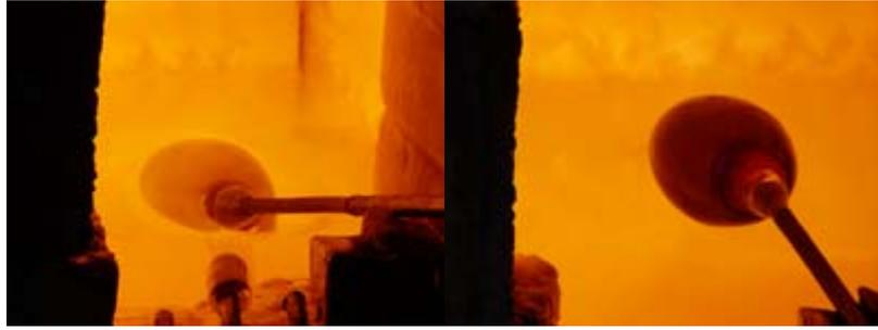
The glassblowers take the glass using a blowing pipe. This process has to be very fast, otherwise the molten glass become cold and the process of inflating cannot take place anymore. Every ball taken from the oven is checked for purity and if the test pass, the ball is inflated until the wanted size is reached.
